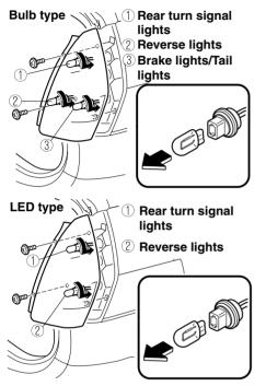
The LED-type bulbs for the brake lights/ taillights/Rear side-marker lights cannot be replaced by the customer. For bulb replacement, consult an Authorized Mazda Dealer.
